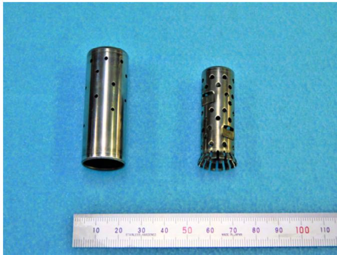
Continual working from deep-drawing to horizontal hole processing by transfer press
